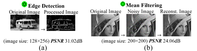
(image size: 128 \times 256 ) PSNR 31.02dB (a) (image size: 200 \times 200 ) PSNR 24.06dB (b) ● \rightarrow N=256 , using circuit topology of [18], w/ optimized library, SLG, total P=10.56mW . ● \rightarrow N=256 , using circuit topology of [20], w/ optimized library, SLG, total P=8.56mW , while w/o optimization P=11.67mW .
